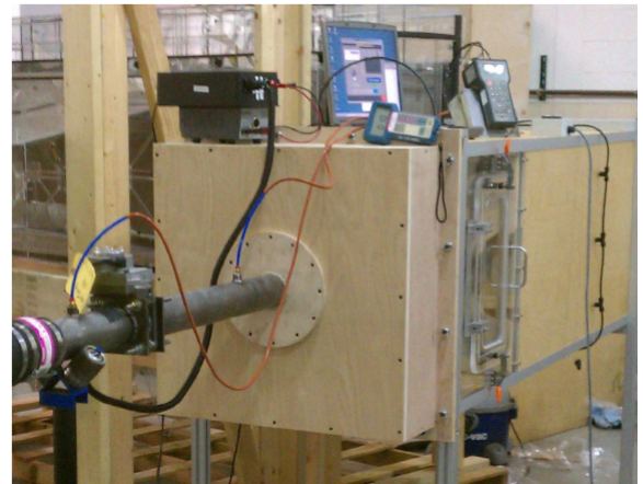
Valve pressure drop test.
