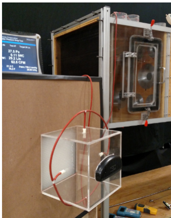
A/C vent pressure drop.
