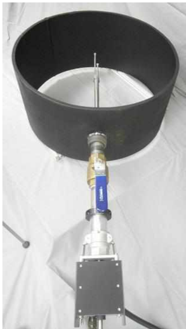
Motorized SwivelSampler mounted on demonstration coal pipe
